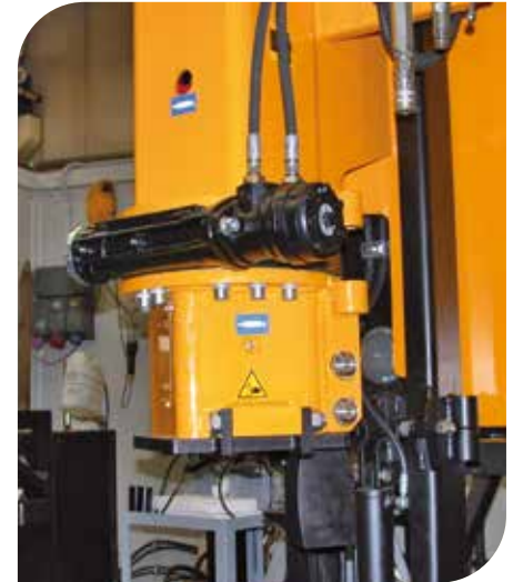
ROTATING HAMMER MOUTH FOR THE ORIENTATION OF THE ANGULAR SQUARED POSTS (accessory)
