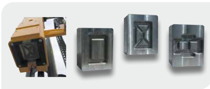
PLATES - Plates of super resistant material with post profiles milling
