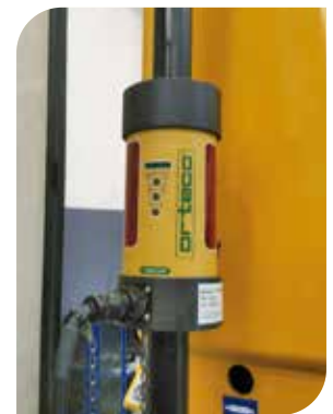
ROTATING HAMMER MOUTH FOR THE ORIENTATION OF THE ANGULAR SQUARED POSTS (accessory)
