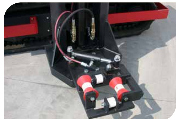
HYDRAULICALLY OPERATED LOWER GUIDE WITH PLASTIC ROLLERS TO PRESERVE THE SURFACES OF THE WOODEN PROFILES (accessory)
