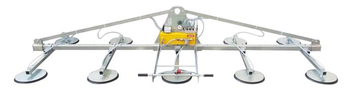
The vacuum lifter for metal sheet **F10A-2000** is a model with compressed air operating system and requires connection to the pneumatic system. The model F10A-2000 has a maximum capacity of 2000 kg, is composed by a crossbar which can be produced in different lengths, on standard models of L3000 mm, L4000 or L5000 mm and 10 suction pads d. 310 mm distributed on 5 arms. **The suction pads**, equipped with springs, are **specific for sheet metal made of special oil-resistant vulcanized rubber**.
