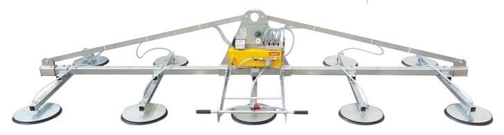
The Vacuum Lifter for sheet metal F10B is a model with **batteries operating system**. The model F10B 3000 has a maximum capacity of 3000 kg, it has a cross-beam which can be made with different lengths, on standard models L3000 mm, L4000 mm or L5000mm and it has 10 suction pads distributed on 5 arms. The pads, equipped with springs, are specific for sheet metal made in **special oil-resistant vulcanized rubber**.
