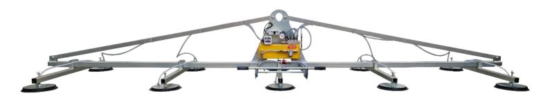
The Vacuum Lifter for sheet metal F10EB is a model with **electric operating system** 400V three-phase or 220V single-phase. The model F10EB 2000 has a maximum capacity of 2000 kg, it has a cross-beam which can be made with different lengths, on standard models L3000 mm, L4000 mm or L5000mm and it has 10 suction pads distributed on 5 arms. The pads, equipped with springs, are specific for sheet metal made in **special oil-resistant vulcanized rubber**.
