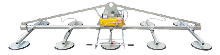
The Vacuum Lifter for sheet metal F10EB is a model with **electric operating system** 400V three-phase or 220V single-phase. The model F10EB 3000 has a maximum capacity of 3000 kg, it has a cross-beam which can be made with different lengths, on standard models L3000 mm, L4000 mm or L5000mm and it has 10 suction pads distributed on 5 arms. The pads, equipped with springs, are specific for sheet metal made in **special oil-resistant vulcanized rubber**.
