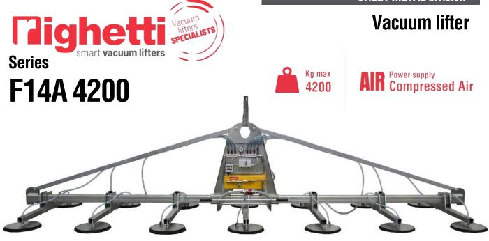
The vacuum lifter for metal sheet **F14A-4200** is a model with compressed air operating system and requires connection to the pneumatic system. The model F14A-4200 has a maximum capacity of 4200 kg, it is composed by a crossbar which can be produced in different lengths and 14 suction pads d. 390 mm distributed on 7 arms. **The suction pads**, equipped with springs, are **specific for sheet metal made of special oil-resistant vulcanized rubber**.
