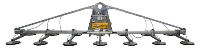
**F14EB 2800** is an electrically powered vacuum lifter, ideal for use on bridge cranes or any other lifting means where it's convenient to get the electrical power supply. The vacuum lifter has a horizontally fixed frame and **14 suction pads**, which are distributed on 7 arms. The length of the arms is at the customer's choice.
