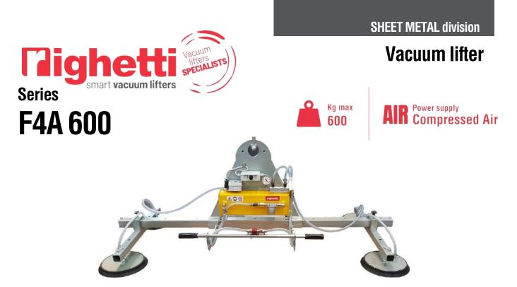
The Vacuum Lifter for metal sheet F4A is a model with **pneumatic operating system**. The model F4A 600 has a maximum capacity of 600 kg and **4 suction pads** distributed on 2 cross-arms. The pads, equipped with springs, are made of **special oil-resistant vulcanized rubber**, specific for sheet metal.
