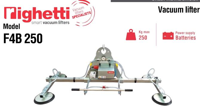
The sheet metal vacuum lifter F4B is battery powered by high capacity rechargeable batteries (battery charger is included). F4B 250 has a maximum capacity of 250 kg and **4 suction pads** distributed on 2 cross-arms. The pads, equipped with springs, are made of **special oil-resistant vulcanized rubber**, specific for sheet metal.
