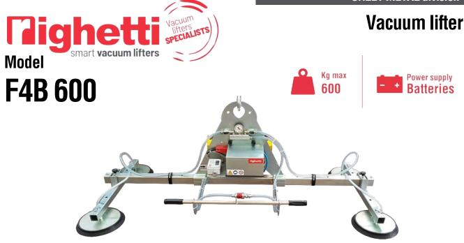
The sheet metal vacuum lifter F4B is battery powered by high capacity rechargeable batteries (battery charger is included). F4B 600 has a maximum capacity of 600 kg and **4 suction pads** distributed on 2 cross-arms. The pads, equipped with springs, are made of **special oil-resistant vulcanized rubber**, specific for sheet metal.
