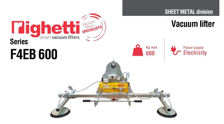
The Vacuum Lifter for metal sheet F4EB is a model with **electric operating system**, it's possible to choose between 400V three-phase or 220V single-phase. The model F4EB 600 has a maximum capacity of 600 kg and **4 suction pads** distributed on 2 cross-arms. The pads, equipped with springs, are made of **special oil-resistant vulcanized rubber**, specific for sheet metal.
