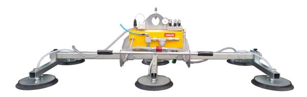
The Vacuum Lifter for sheets metal **F6A 1800** is a model with compressed air operating system and requires connection to the pneumatic system. The model F6A 1800 has a maximum capacity of 1800 kg and **6 suction pads** distributed on 3 cross-arms. The pads, equipped with springs, are made of **special oil-resistant vulcanized rubber**, specific for sheet metal. The lifter can be produced with different crossbeam lengths, from L1500 mm to L4000 mm (different lengths on request).
