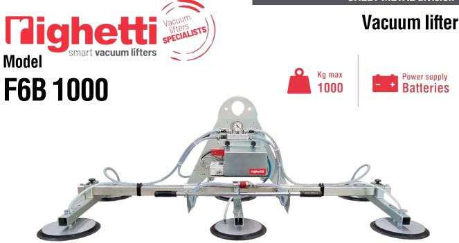
The sheet metal vacuum lifter F6B is battery powered by high capacity rechargeable batteries (battery charger is included). F6B 1000 has a maximum capacity of 1000 kg and **6 suction pads** distributed on 3 cross-arms. The pads, equipped with springs, are made of **special oil-resistant vulcanized rubber**, specific for sheet metal.
