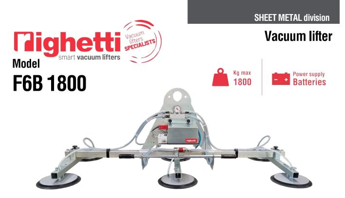
The sheet metal vacuum lifter F6B is battery powered by high capacity rechargeable batteries (battery charger is included). F6B 1800 has a maximum capacity of 1800 kg and **6 suction pads** distributed on 3 cross-arms. The pads, equipped with springs, are made of **special oil-resistant vulcanized rubber**, specific for sheet metal.
