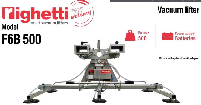
The sheet metal vacuum lifter F6B is battery powered by high capacity rechargeable batteries (battery charger is included). F6B 500 has a maximum capacity of 500 kg and **6 suction pads** distributed on 3 cross-arms. The pads, equipped with springs, are made of **special oil-resistant vulcanized rubber**, specific for sheet metal.
