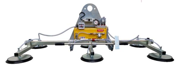
The Vacuum Lifter for metal sheet F6EB is a model with **electric operating system**, it's possible to choose between 400V three-phase or 220V single-phase. The model F6EB 1000 has a maximum capacity of 1000 kg and **6 suction pads** distributed on 3 cross-arms. The pads, equipped with springs, are made of **special oil-resistant vulcanized rubber**, specific for sheet metal.
