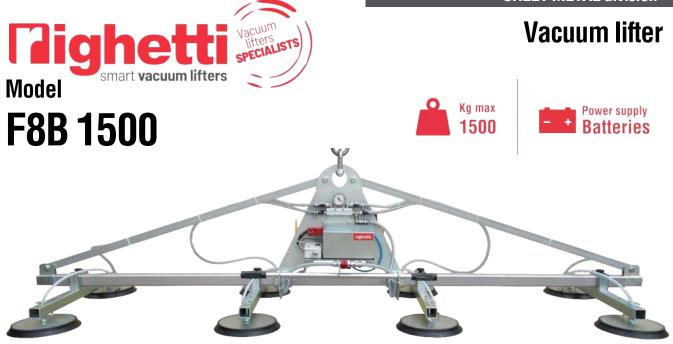
The sheet metal vacuum lifter F8B is battery powered by high capacity rechargeable batteries (battery charger is included). F8B 1500 has a maximum capacity of 1500 kg and 8 **suction pads** distributed on 4 cross-arms. The pads, equipped with springs, are made of **special oil-resistant vulcanized rubber**, specific for sheet metal.
