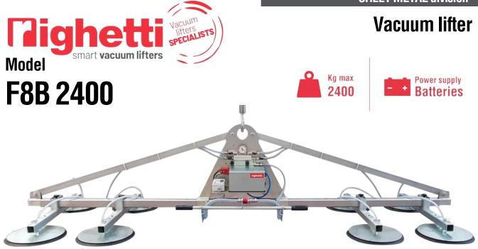
The sheet metal vacuum lifter F8B is battery powered by high capacity rechargeable batteries (battery charger is included). F8B 2400 has a maximum capacity of 2400 kg and 8 suction pads distributed on 4 cross-arms. The pads, equipped with springs, are made of **special oil-resistant vulcanized rubber**, specific for sheet metal.
