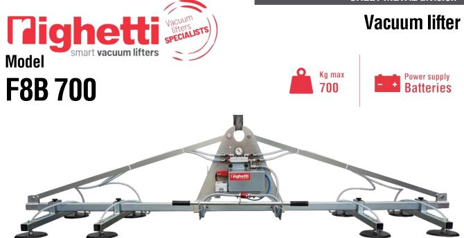
The sheet metal vacuum lifter F8B is battery powered by high capacity rechargeable batteries (battery charger is included). F8B 700 has a maximum capacity of 700 kg and 8 **suction pads** distributed on 4 cross-arms. The pads, equipped with springs, are made of **special oil-resistant vulcanized rubber**, specific for sheet metal.
