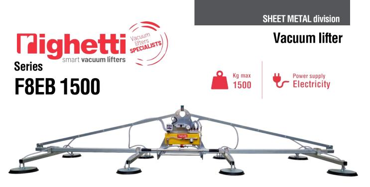
The Vacuum Lifter for sheet metal F8EB is a model with **electric operating system**, it can be produced 400V three-phase or 220V single-phase. The model F8EB 1500 has a maximum capacity of 1500 kg. The **crossbeam can have different lengths**, on standard models it is L3000 mm or L4000 mm and the 8 suction pads are distributed on 4 arms. The pads, equipped with springs, are specific for sheet metal made in **special oil-resistant vulcanized rubber**.
