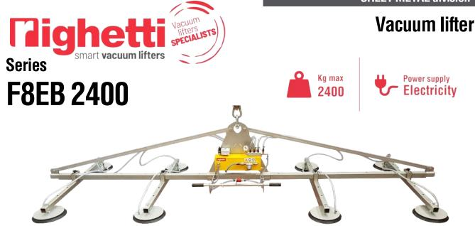
The Vacuum Lifter for sheet metal F8EB is a model with **electric operating system**, it can be produced 400V three-phase or 220V single-phase. The model F8EB 2400 has a maximum capacity of 2400 kg. The **crossbeam can have different lengths**, on standard models it is L3000 mm or L4000 mm and the 8 suction pads are distributed on 4 arms. The pads, equipped with springs, are specific for sheet metal made in **special oil-resistant vulcanized rubber**.
