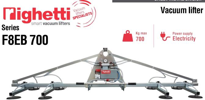
The Vacuum Lifter for sheet metal F8EB is a model with **electric operating system**, it can be produced 400V three-phase or 220V single-phase. The model F8EB 700 has a maximum capacity of 700 kg. The **crossbeam can have different lengths**, on standard models it is L3000 mm or L4000 mm and the 8 suction pads are distributed on 4 arms. The pads, equipped with springs, are specific for sheet metal made in **special oil-resistant vulcanized rubber**.
