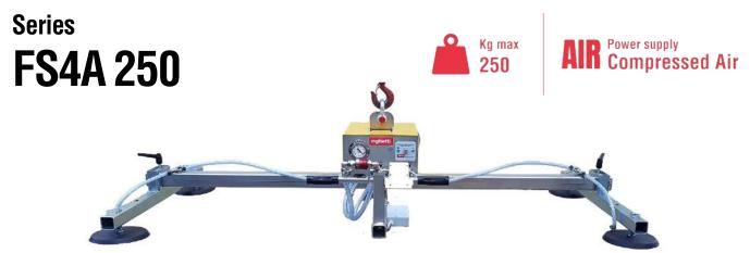
The Vacuum Lifter for sheets metal **FS4A 250** is a model with compressed air operating system and requires connection to the pneumatic system. The model FS4A 250 has a maximum capacity of 250 kg and **4 suction pads** distributed on 2 cross-arms. The pads, equipped with springs, are made of **special oil-resistant vulcanized rubber**, specific for sheet metal.
