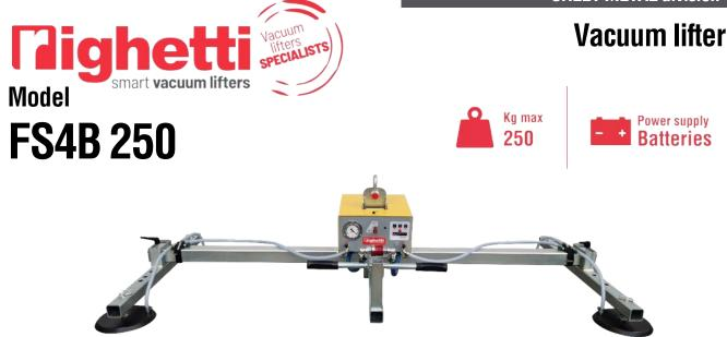
The sheet metal vacuum lifter FS4B is battery powered by high capacity rechargeable batteries (battery charger is included). FS4B has a maximum capacity of 250 kg and **4 suction pads** distributed on 2 cross-arms. The pads, equipped with springs, are made of **special oil-resistant vulcanized rubber**, specific for sheet metal.
