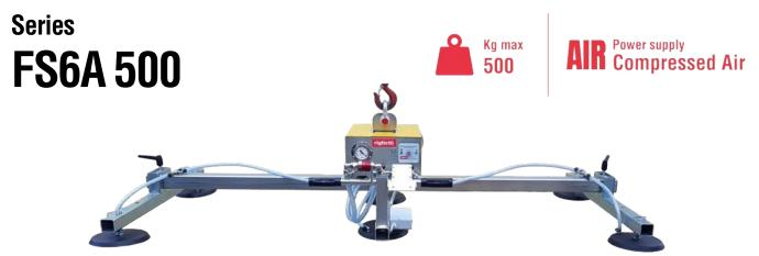
The Vacuum Lifter for sheets metal **FS6A 500** is a model with compressed air operating system and requires connection to the pneumatic system. The model FS6A 500 has a maximum capacity of 500 kg and **6 suction pads** distributed on 3 cross-arms. The pads, equipped with springs, are made of **special oil-resistant vulcanized rubber**, specific for sheet metal.
