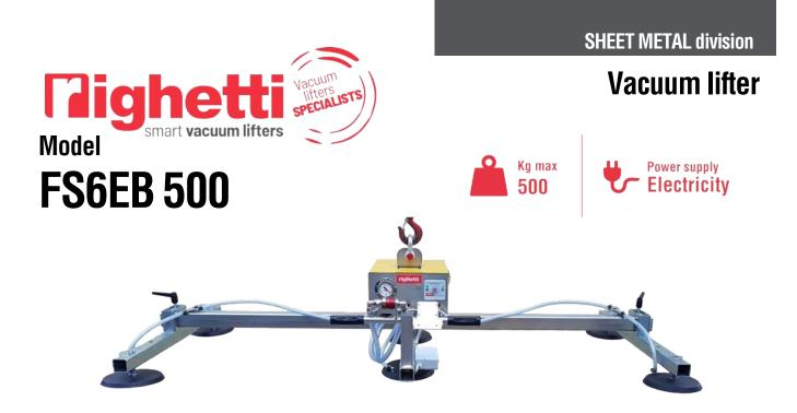
The Vacuum Lifter for sheet metal **FS6 EB 500** is an electric powered model. It is possible to choose between 400V threephase or 220V single-phase. The pads, equipped with springs, are made of **special oil-resistant vulcanized rubber**, specific for sheet metal.
