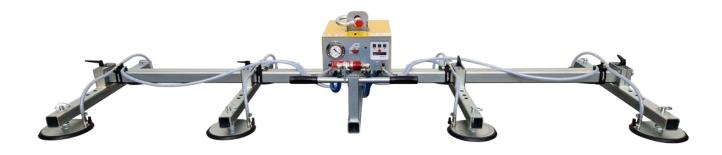
The Vacuum Lifter for sheet metal **FS8 EB 600** is an electric powered model. It is possible to choose between 400V three-phase or 220V single-phase. The pads, equipped with springs, are made of **special oil-resistant vulcanized rubber**, specific for sheet metal.
