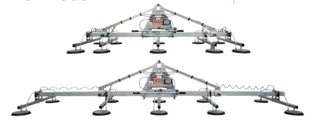
**FT10A1800** is a sheet metal vacuum lifter with telescopic frame. Being its **length adjustable from 2900mm to 5120mm**, it is the perfect vacuum lifter for handling **sheet metal of all the standard dimension** (**6000x2000**mm – **4000x2000**mm – **3000x1500**mm). Moreover, FT10A1800 comes equipped with the possibility of arms shut-off by a tap positioned on the lifter frame.
