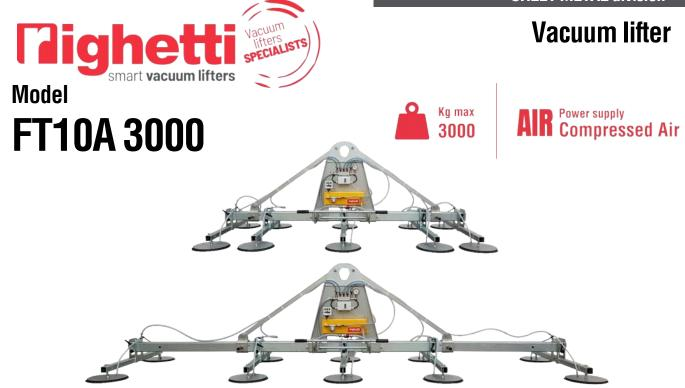
**FT10A3000** is a sheet metal vacuum lifter with telescopic frame. Being its **length adjustable from 2860mm to 5000mm**, it is the perfect vacuum lifter for handling **sheet metal of all the standard dimension** (**6000x2000**mm – **4000x2000**mm – **3000x1500**mm). Moreover, FT10A3000 comes equipped with the possibility of arms shut-off by a tap positioned on the lifter frame.
