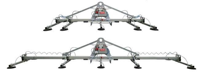
**FT10A800** is a sheet metal vacuum lifter with telescopic frame. Being its **length adjustable from 2651mm to 4897mm**, it is the perfect vacuum lifter for handling **sheet metal of all the standard dimension** (**6000x2000**mm – **4000x2000**mm – **3000x1500**mm). Moreover, FT10A800 comes equipped with the possibility of arms shut-off by a tap positioned on the lifter frame.
