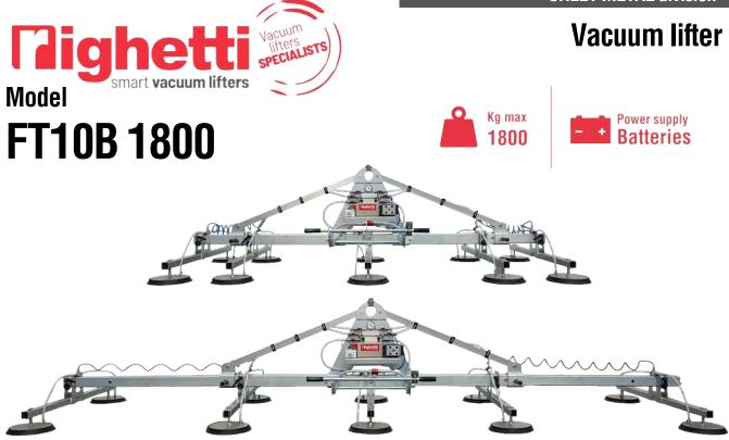
**FT10B1800** is a sheet metal vacuum lifter with **telescopic frame**. Being **its length adjustable** from 2761mm to 5007mm, it is the perfect vacuum lifter for handling sheet metal of variable dimensions such as 6000x2000mm, 4000x2000mm and 3000x1500mm. Moreover, FT10B1800 comes equipped with the possibility of **excluding arms** from suction by simply switching off a tap.
