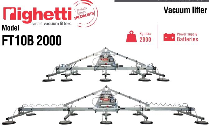
**FT10B2000** is a sheet metal vacuum lifter with **telescopic frame**. Being **its length adjustable** from 2761mm to 5007mm, it is the perfect vacuum lifter for handling sheet metal of variable dimensions such as 6000x2000mm, 4000x2000mm and 3000x1500mm. Moreover, FT10B2000 comes equipped with the possibility of **excluding arms** from suction by simply switching off a tap.
