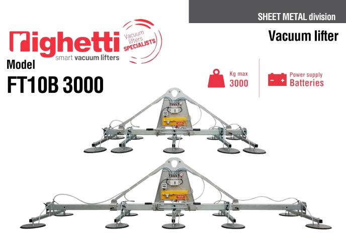
**FT10B3000** is a sheet metal vacuum lifter with **telescopic frame**. Being **its length adjustable** from 2860mm to 5000mm, it is the perfect vacuum lifter for handling sheet metal of variable dimensions such as 6000x2000mm, 4000x2000mm and 3000x1500mm. Moreover, FT10B3000 comes equipped with the possibility of **excluding arms** from suction by simply switching off a tap.
