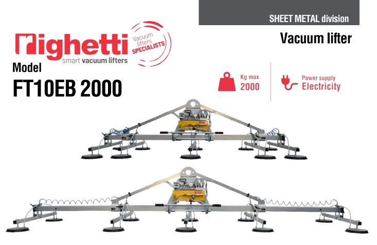
**FT10EB2000** is a sheet metal vacuum lifter with **telescopic frame**. Being **its length adjustable** from 2761 mm to 5007 mm, it is the perfect vacuum lifter for handling sheet metal of variable dimensions such as 6000x2000mm, 4000x2000mm and 3000x1500mm. Moreover, FT10EB2000 comes equipped with the possibility of **excluding arms** from suction by simply switching off a tap.
