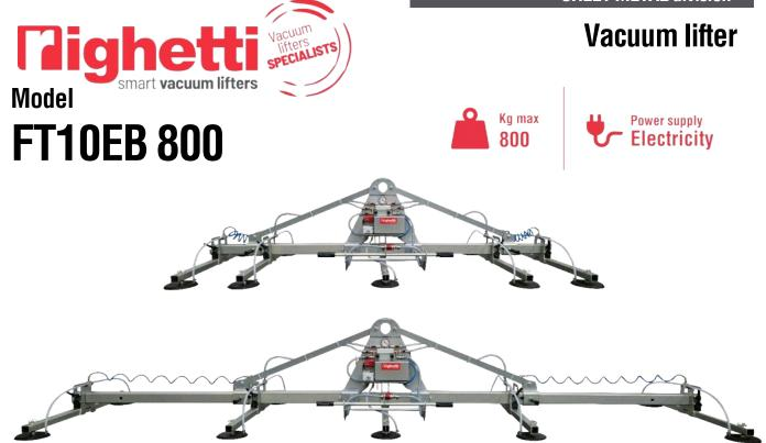
**FT10EB800** is a sheet metal vacuum lifter with **telescopic frame**. Being **its length adjustable** from 2651mm to 4897mm, it is the perfect vacuum lifter for handling sheet metal of variable dimensions such as 6000x2000mm, 4000x2000mm and 3000x1500mm. Moreover, FT10EB800 comes equipped with the possibility of **excluding arms** from suction by simply switching off a tap.
