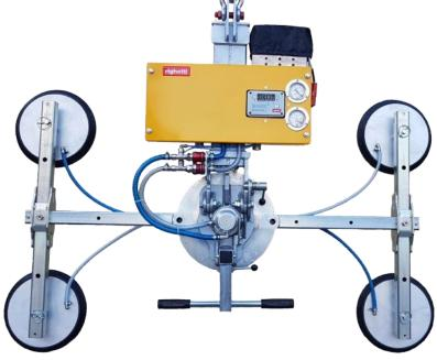
GL-VB4TR vacuum glass lifter is a modular vacuum lifter. Along the 1500mm long central beam, the 4 suction pads can be placed both on cross arms or in a row on the main beam. In any case, suction pads are repositionable on the arms, which are movable as well along the central beam.
