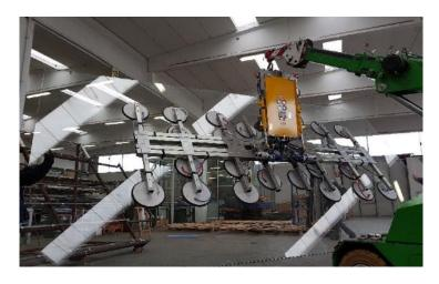
GLE3000 is a modular vacuum lifter with lifting capacity up to 3000 Kg, perfect for big and heavy glass installations. GLE3000 has continuous 360° electric rotation and 0 - 90° electric tilt. It has battery operating system with rechargeable batteries that, if necessary, may be easily removed and quickly replaced.
