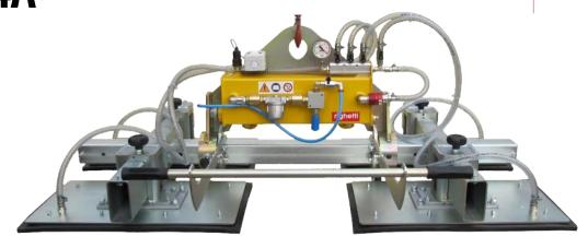
The M4A is a series of vacuum lifters which contains a wide range of 4-plates models with capacities ranging from 500 kg to 2000 kg. The M4A series is compressed air powered. The **manual tilting system** allows a vertical – horizontal movement and vice versa. The maximum capacity of the lift depends on the size of the suction plates.
