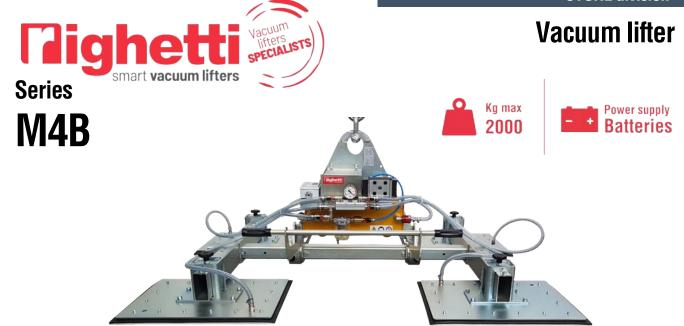
The M4B is a series of Vacuum Lifters which contains a wide range of 4-plates models with capacities ranging from 500 kg to 2000 kg. The M4B series is powered by on board, rechargeable and long lasting batteries. The battery charger is included. The manual tilting system allows a vertical – horizontal movement and vice versa. The maximum capacity of the lift depends on the size of the suction plates.
