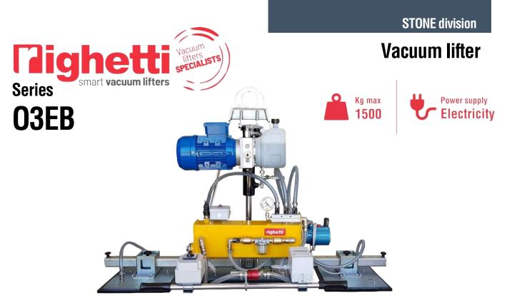
The O3EB is a series of Vacuum Lifters which contains a wide range of 3-plates models with **capacities ranging from 375 kg to 1500 kg**. The O3EB series is electric powered and it can be produced with voltage 220V 1phase or 400V 3phases. The **hydraulic tilting** system allows a powered vertical – horizontal movement and vice versa; controlled by an electric switch, placed on the lifter's handle.
