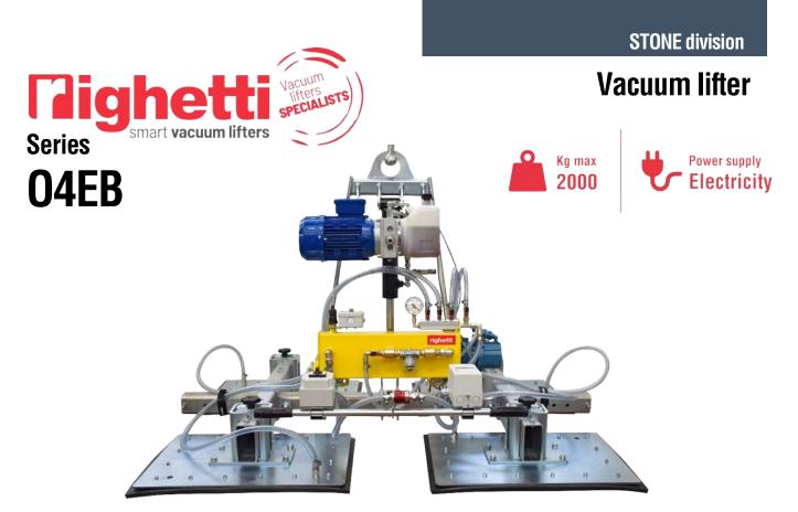
The O4EB is a series of Vacuum Lifters which contains a wide range of 4-plate models with **capacities ranging from 500 kg to 2000 kg**. The O4EB series is electric powered and it can be produced with voltage 220V 1phase or 400V 3phases. The oil **hydraulic tilting** system allows a powered vertical – horizontal movement and vice versa; controlled by an electric switch, placed on the lifter's handle.
