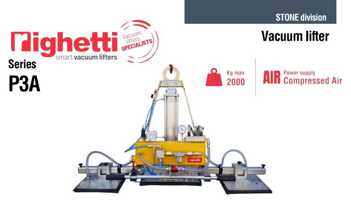
The P3A series of Vacuum Lifters is a range of 3-pads models with lifting capacity **from 375 kg to 2000 kg**. The P3A series is powered by compressed air. The **pneumatic tilting system** allows an assisted movement vertical – horizontal of the load and vice versa. The maximum capacity of the lifter depends on the dimension of the suction plates.
