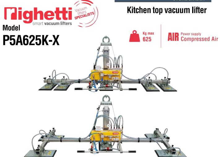
The model P5A625K-X is a **transformable vacuum lifter** with 5 pads and lifting capacity **625 kg**. Thanks to two extension arms (L 830mm), this lifter can change configuration from inline-pads, **suitable for kitchen tops**, to cross-pads, **suitable for big slabs**. The standard central beam is 2400mm long. All the 5 vacuum pads feature **support for quick rotation**.
