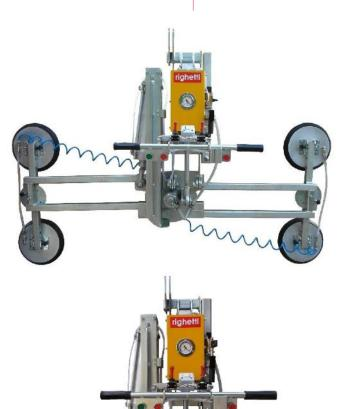
The model R1 is a versatile and professional **vacuum glass lifter specific for use in production**, with four suction pads d. 310 mm, compressed air powered and lifting capacity 400Kg. Thank to its two pneumatic cylinders, the R1 features **pneumatic 90° rotation and pneumatic 90° tilt**, controlled with two joysticks placed on the lifter's handle. It has pneumatic buttons to command suction and release.
