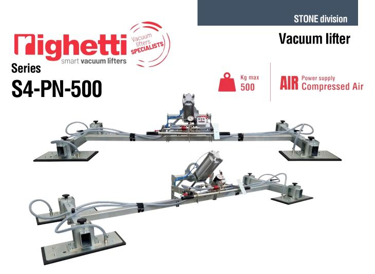
The S4-PN is a series of pneumatic vacuum stone lifters with **lowered frame** and lifting capacity 500kg. The **tilting system is powered by a pneumatic cylinder** which allows the movement of the load from vertical to horizontal and vice-versa. It has 4 rectangular vacuum pads mm 480x230.
