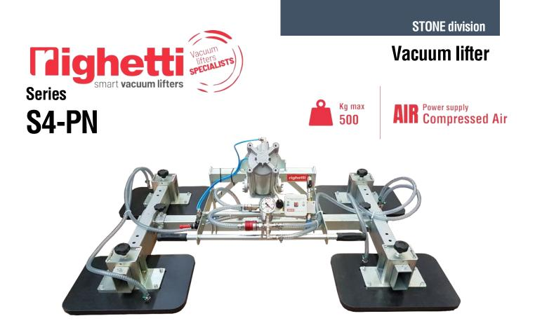
The S4-PN is a series of pneumatic vacuum stone lifters with **lowered frame** and lifting capacity 500kg. The **tilting system is powered by a pneumatic cylinder** which allows the movement of the load from vertical to horizontal and vice-versa. It has 4 rectangular vacuum pads mm 480x230.
