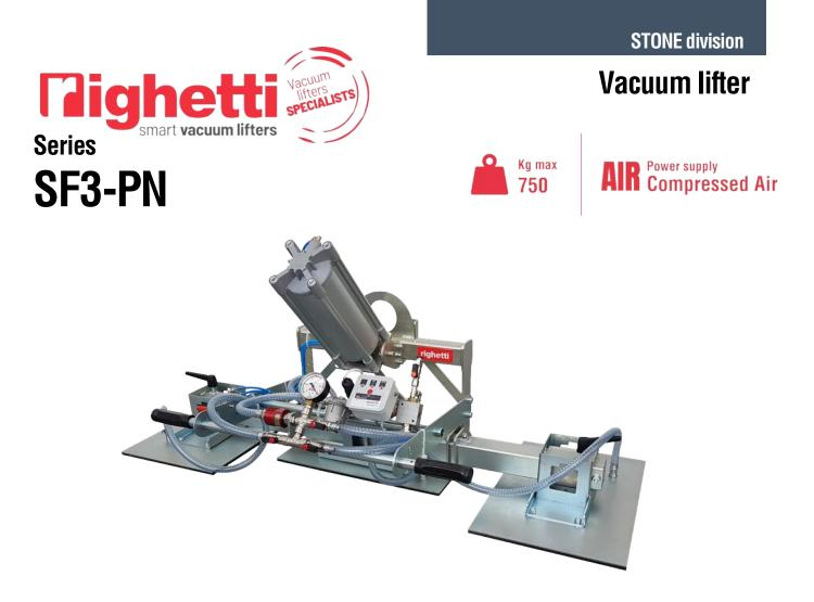
The SF3-PN is a series of pneumatic vacuum stone lifters with **lowered frame** and lifting capacity from 375kg up to 750kg. The **tilting system is powered by a pneumatic cylinder** which allows the movement of the load from vertical to horizontal and vice-versa. This lifter is very versatile, by excluding the side plates by turning off a tap on the lifter's frame, it is possible to **use only the central plate** that allows you to lift small items.
