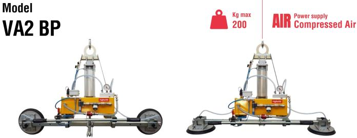
The model VA2 BP is a glass vacuum lifter specific **for indoor use**, with two suction pads d. 310 mm, compressed air powered and a lifting capacity up to 200Kg. The pads are movable along the beam in three different positions. The standard central beam is 1500mm long, but different lengths are available on request.
