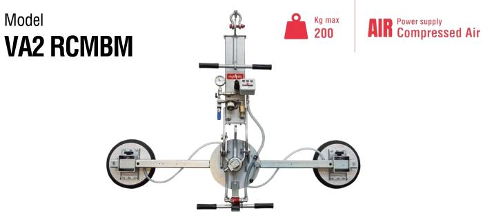
The model VA2 RCMBM is a **vacuum glass lifter specific for indoor use**, with two suction pads d. 310 mm, compressed air powered with lifting capacity up to 200Kg. The pads are replaceable along the arms in different positions.
