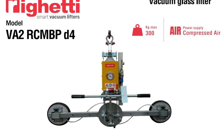
The model VA2 RCMBP d4 is a vacuum glass lifter specific for indoor use, with two suction pads d. 390 mm, compressed air powered with lifting capacity up to 300Kg. The pads are replaceable along the beam in different positions. The standard central beam is 1500mm long, on request different lengths.
